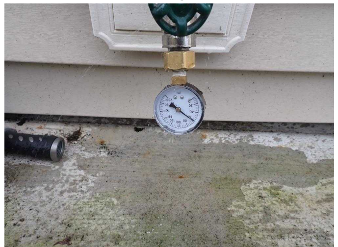
#12 Water pressure tested at 60 psi.
